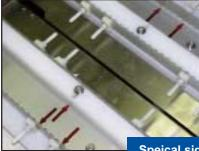
Speical side pins capture the product to hold it in position as it is transfered through the wrapper to the end sealers.
