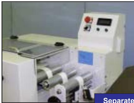
Separate AC motors drive the card stock roll and knife. A dancer roll and brake control card feed tension.
