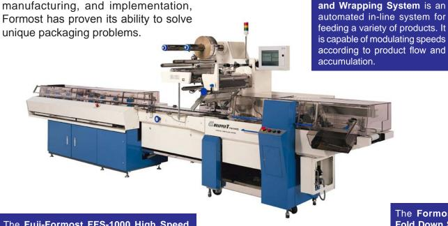
The Fuji-Formost FFS-1000 High Speed Infeed has a multiple belt conveyor system with automatic control of each belt according to product delivery. Shown below with Formost product alignment system. Complete system with Formost Transpositor on front cover.
