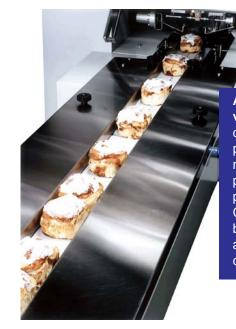
Attachless Infeed Conveyor automatically indexes soft and sticky products into a Fuji-Formost horizontal wrapper at speeds up to 120 packages per minute. Computer controlled flat belts have no lugs and are easy to remove and clean.
