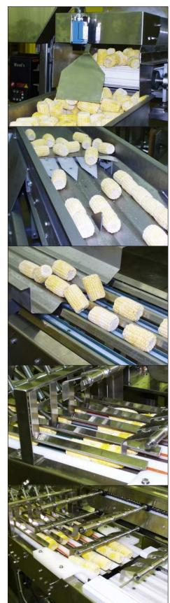
Product is collated on the shaker table and the high-speed accumulation conveyor. Corn is aligned and separated into lanes and the accumulation conveyor accelerates the corn away from the shaker table. The corn is then timed into the wrapper flights by the grouper assembly.
